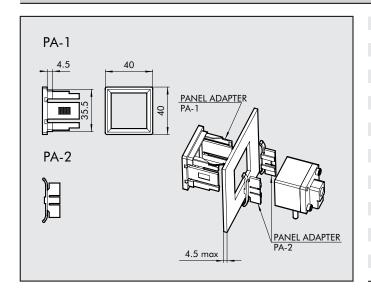
Description 9000602 KIT FOR PANEL FIXING FOR THE DIGITAL PRESSURE SWITCH
