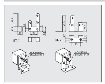
Code Description 9000601 KIT OF FIXING BRACKETS FOR DIGITAL PRESSURE SWITCHES
